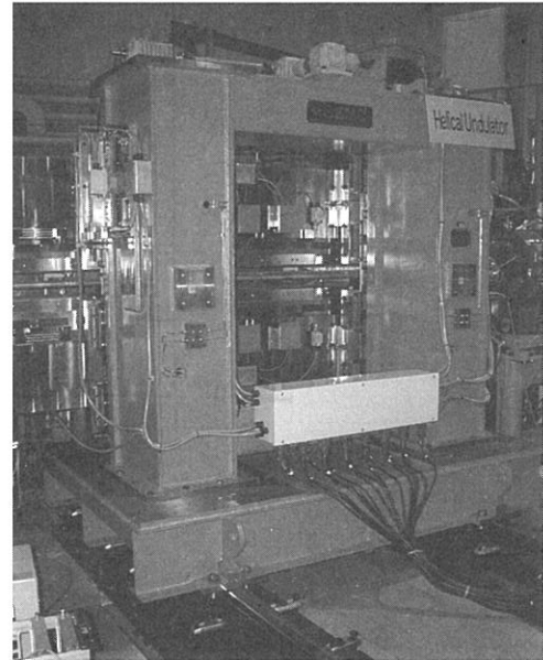
BL5A Helical Undulator (Optical Klystron for FEL)
